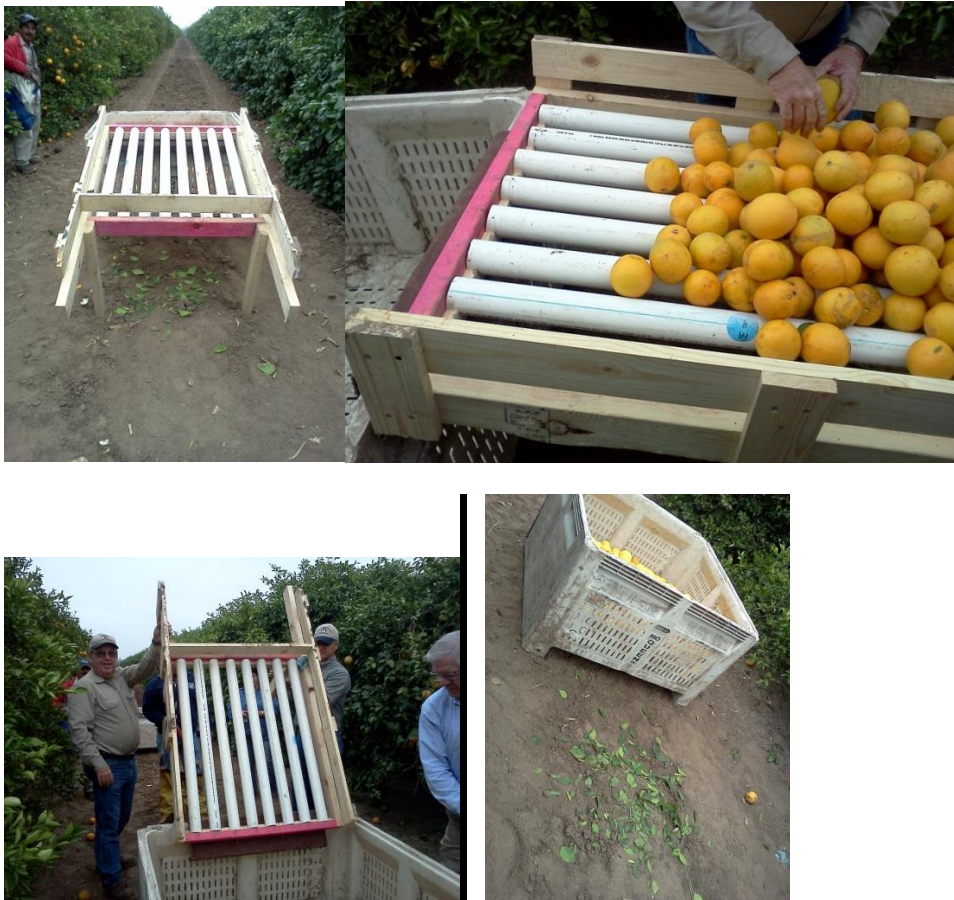
Figure 1. Leaf decontamination table to remove leaves and twigs from harvested fruit before being put into bins.
